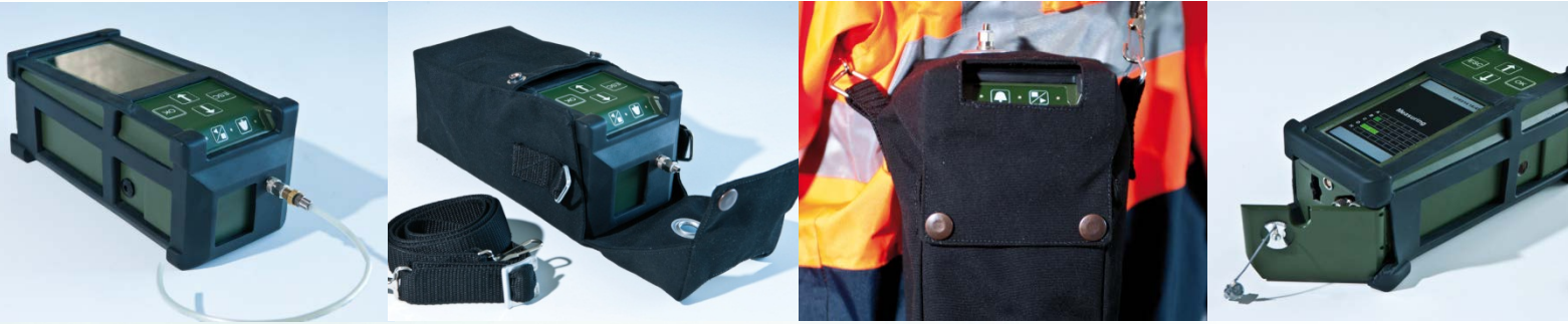
Various supplies: inlet tubing / w filter, bottom and side service covers with dopant cartridge, carrying pouch offers basic operational access
