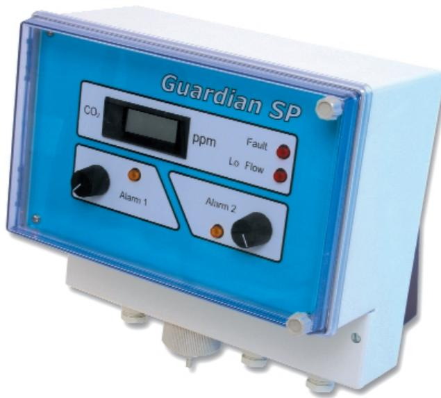
The Guardian range of infrared gas monitors offers near-analyser quality continuous sampling, measurement and display of target gas concentrations at an attractive price.
