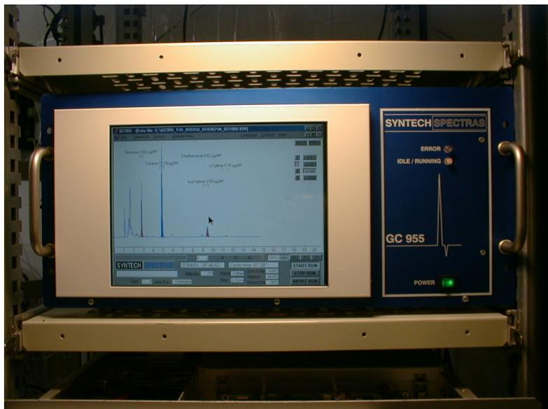
The instrument is a gaschromatograph with a built-in preconcentration system. Hydrocarbons are preconcentrated on Tenax GR, desorbed thermally and separated on an EPA624 equivalent column, to reach optimal separation from interfering hydrocarbons. Analysis is done by a photo ionisation detector and a flame ionisation detector. This ensures high sensitivity and good identification. (For use as a BTX monitor a photo ionisation detector is sufficient, so a cheaper GC855 can be used).
